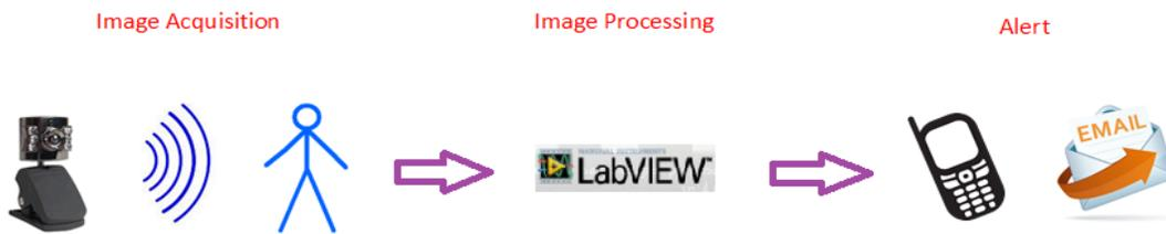
Figure 2. Structure and data flow of Intruder Detection System. Processing occurs in three steps: signal acquisition, signal processing, and alert.
