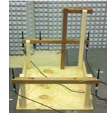
Rig allows for microphones to be offset 1 foot from the center in the y direction, 1 foot or 6 inches in the x direction, and 1 foot or 2 feet in the z direction
