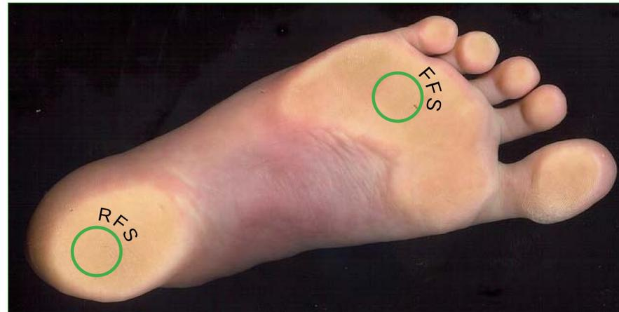
Shown above are the ideal locations for sensor placement. The fore-foot sensor is placed underneath the fourth metatarsal head. By summing the data from the two sensors, we were able to capture an accurate proportional picture of impact force.
