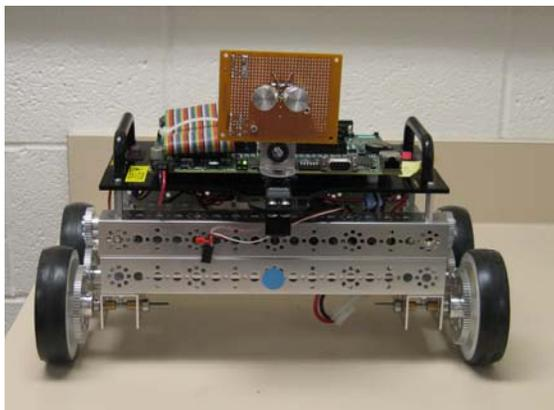
Figure: Photograph of the robot platform used to develop the algorithm. Ultrasonic sensors are visibly attached to a rotating servo motor to allow rotational freedom of motion. The angle of the ultrasonic source relative to the robot is determined by rotating the array until the signals from the two sensors have the same amplitude.
