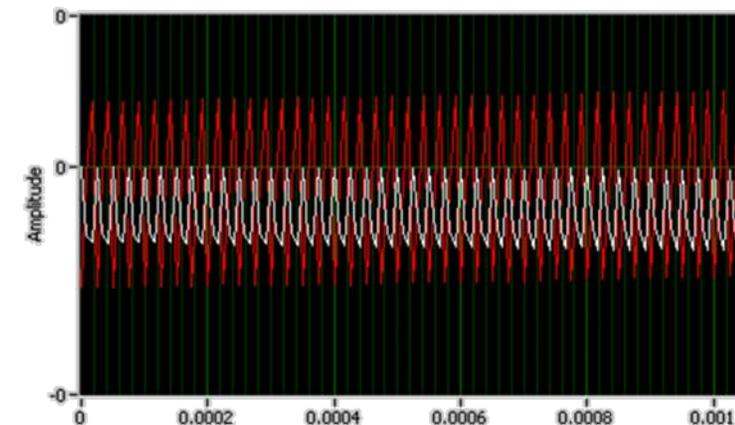
40kHz sinusoid signals received by the two-sensor array. The sensor on the right is represented by the red waveform. Since the amplitude is higher for the right sensor than the left sensor, the target is located toward the right.
