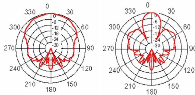
Beam pattern of the ultrasonic transmitter (left) and the receiver (right).
