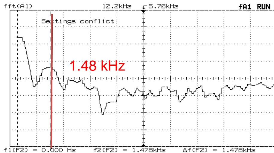
Figure 1: Fast Fourier Analysis of Plug Signal at Approximately 1000 RPM
