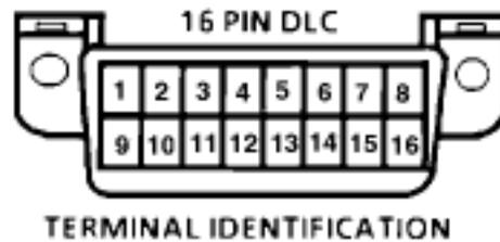
Figure 4: Pin Layout of OBD-II Connector
