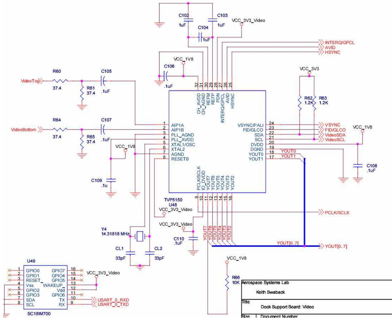
Figure 7 – NTSC Decoder Circuit
