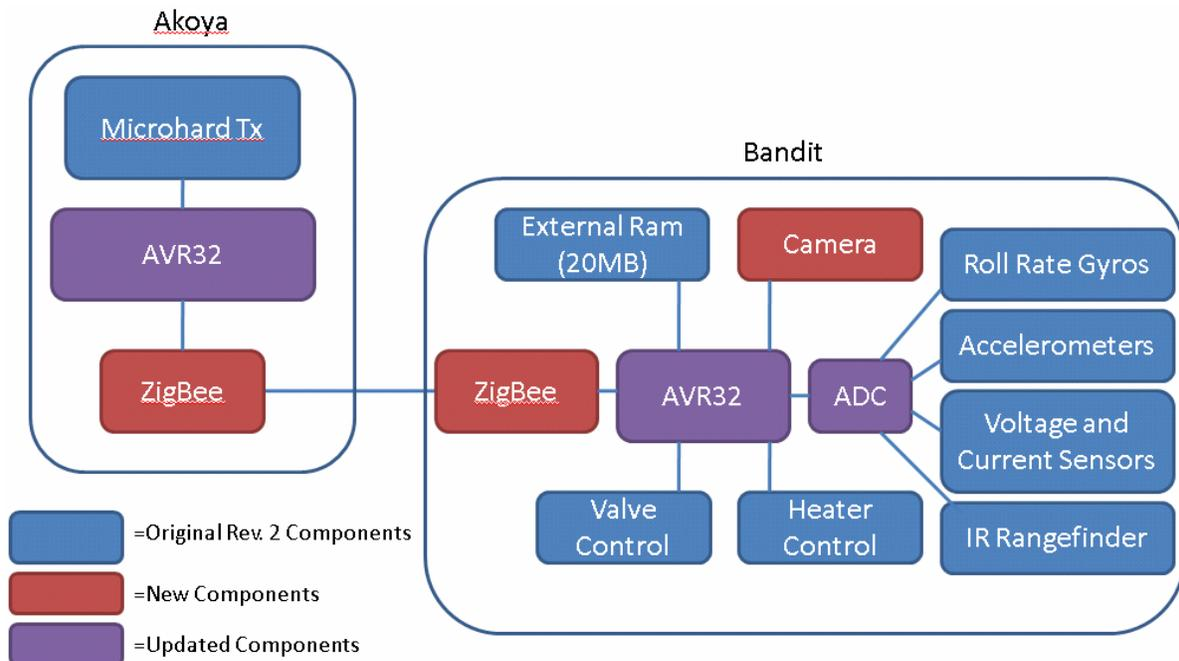
Figure 5 – Changes to Bandit Electronics
