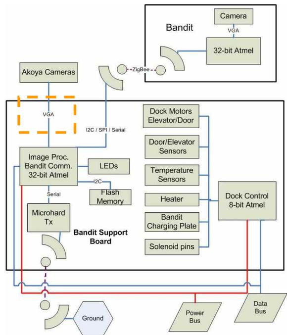
**Figure 4 - Suggested Revision 3 Dock Support Board Block Diagram**
