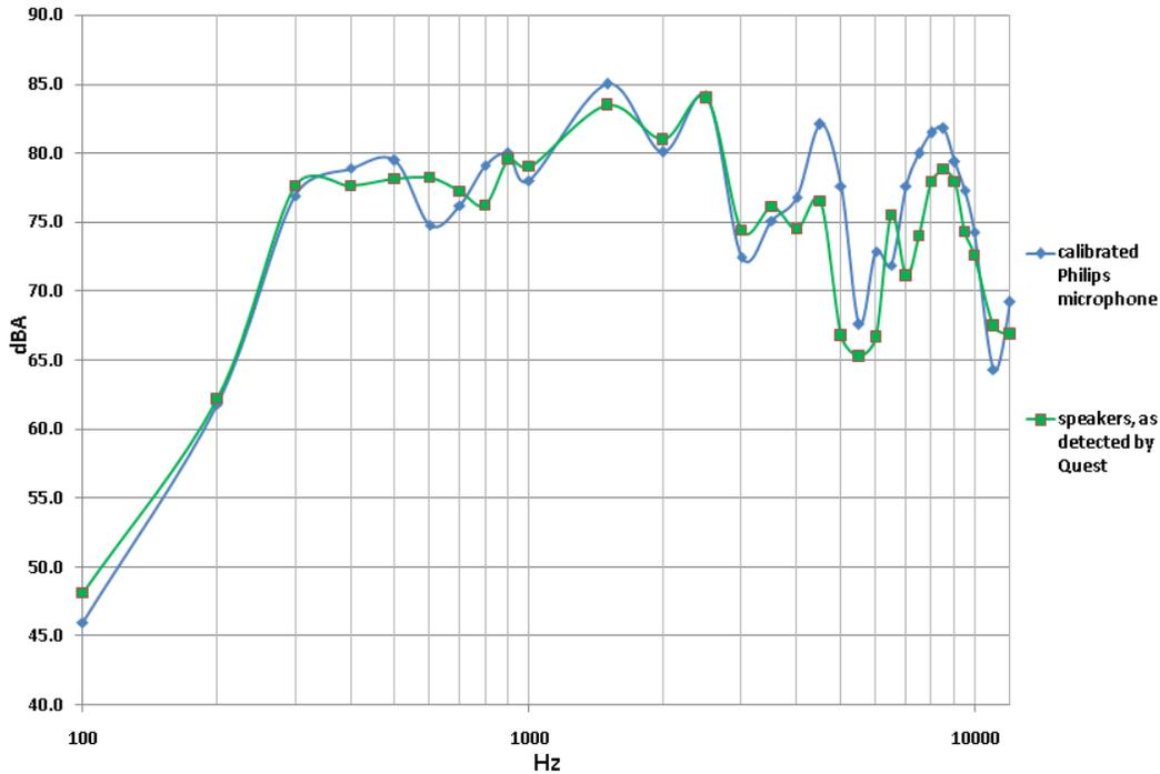
**FIGURE 7** frequency response curves (A-weighted) of microphone with Matlab's calibration constants and speakers
