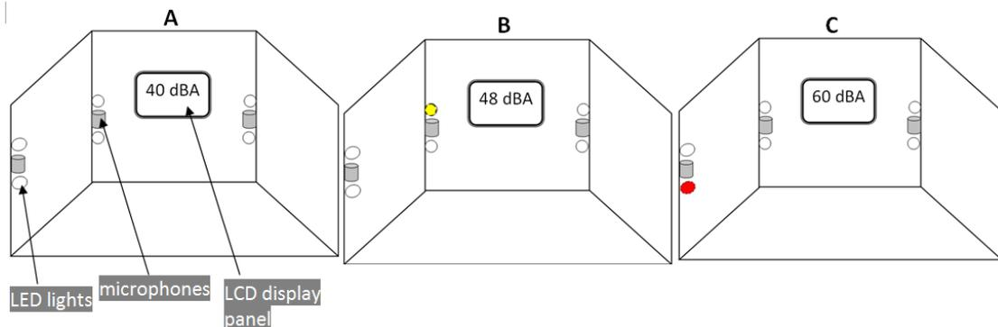
**Figure 10** Sound Level Alarm mock up. Note that figure is not to scale
