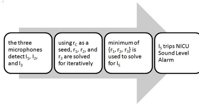
**FIGURE 9** determination of  $I_s$ , sound intensity at the source
