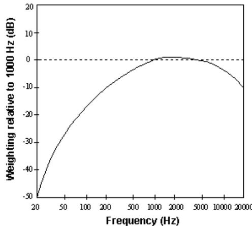
**FIGURE 3** A-weighting filter relative frequency response curve<sup>[6]</sup>
