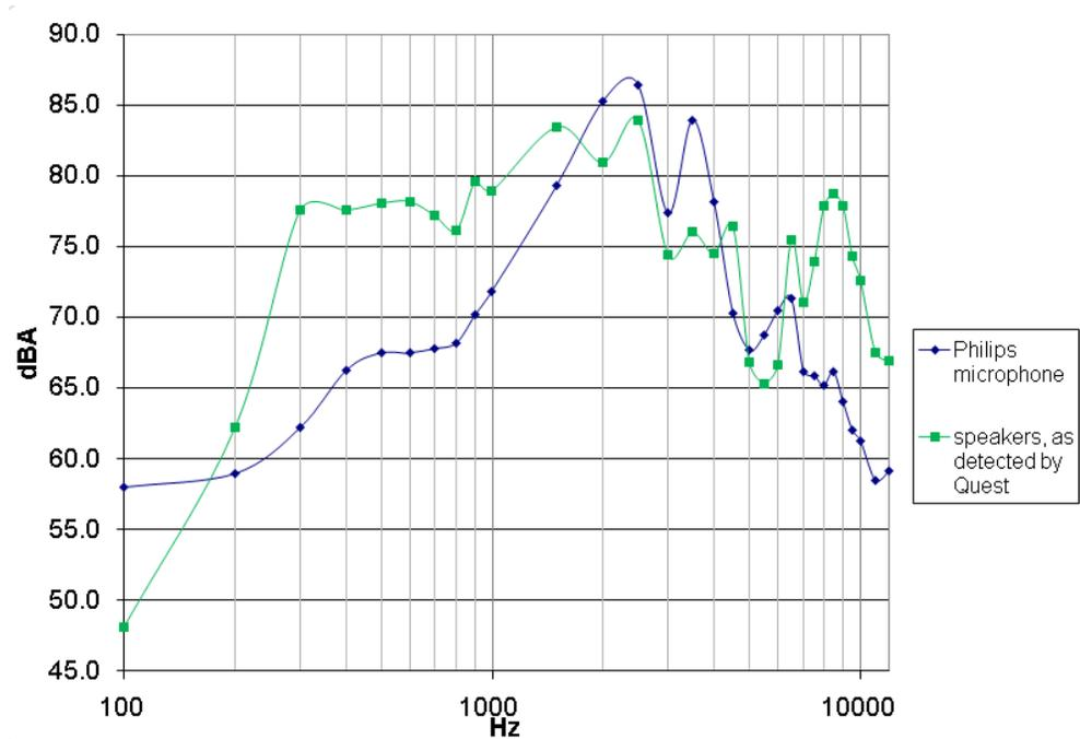
**FIGURE 6** frequency response curves (A-weighted) of microphone and speakers
