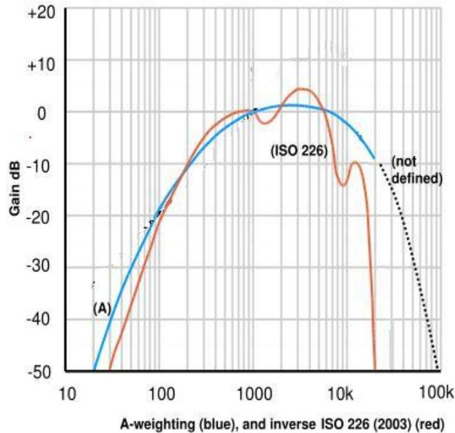
**FIGURE 15** relative dB gain of A-weighting filter and ISO226<sup>[13]</sup>
