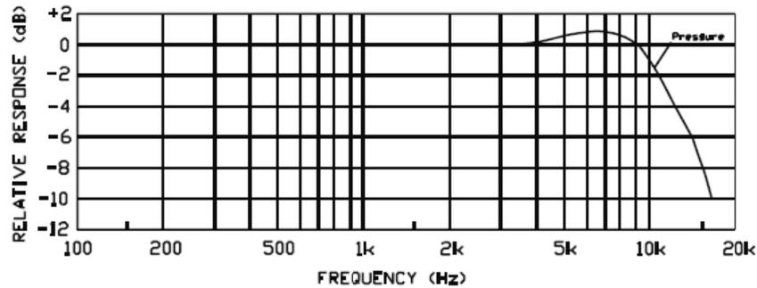
**Figure 5** frequency response curve of the Quest QE4170 microphone<sup>[8]</sup>
