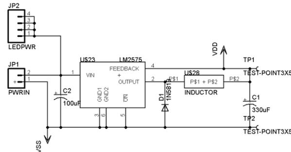
Fig. 6. The switching regulator circuit as implemented in EAGLE<sup>®</sup> with an LM2575-3.3 regulator.
