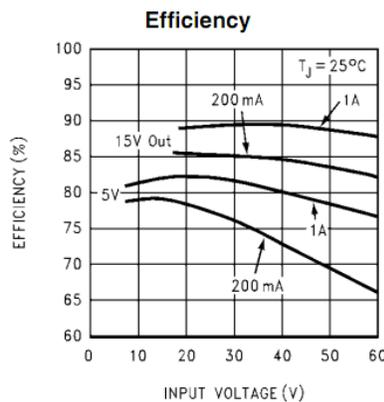
Fig. 7. Typical efficiency curves of an LM2575-3.3 regulator as provided by the manufacturer [11]. Extrapolation from the graph suggests a typical efficiency of about 75% for 3.3 V, 375 mA output and 9V input.
