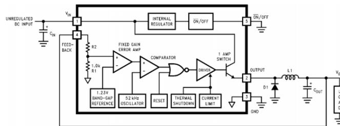
Fig. 4. Block diagram of the LM2575 step-down switching regulator as shown in the product datasheet [11]. The LM2575 implements the switching and negative feedback functions of the black box in the simplified schematic in Fig. 3.
