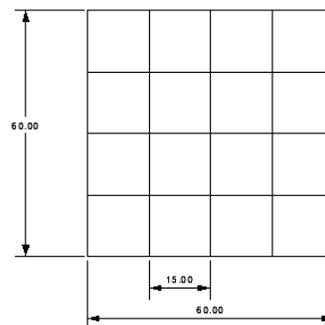
Fig. 1. Physical layout of a single module. Each module is 60 cm by 60 cm and has 16 pixels driven by four RGBW LEDs each.
