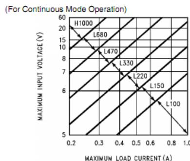
Fig. 5. Inductor values recommended by National Semiconductor in the LM2575 datasheet [11].
