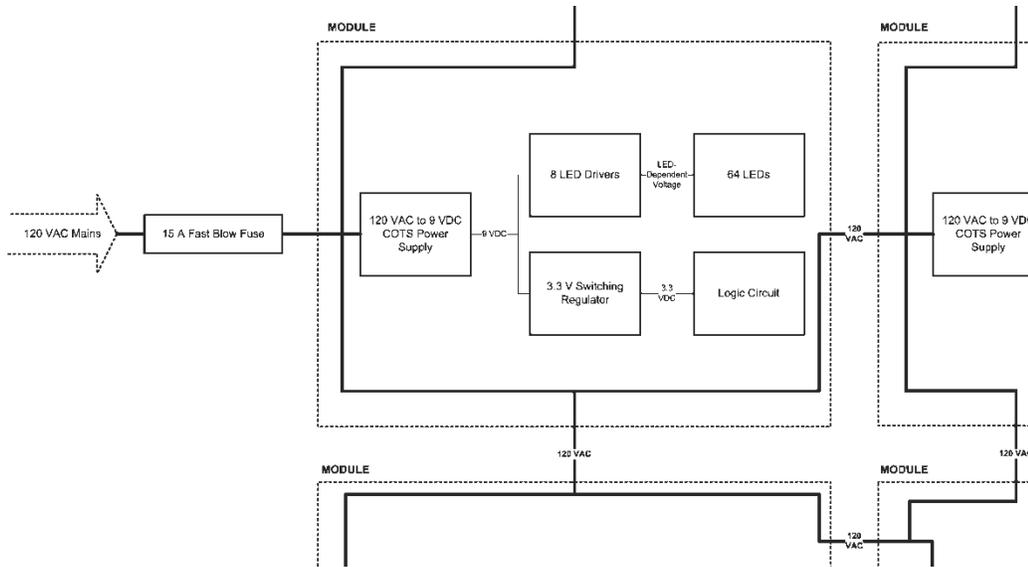
Fig. 10. Block diagram of the entire dance floor power distribution and regulation system. The diagram shows how the modules are interconnected and how the modules internally regulate power for the various devices.
