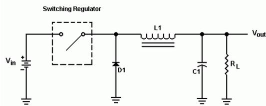
Fig. 3. Schematic diagram of a simple step-down switching regulator [10]. The regulator “switches” the power supply relying on stored energy in passive components which results in high efficiencies.
