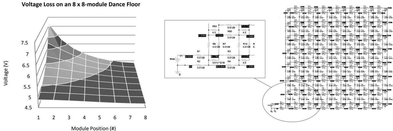
Fig. 9. PSpice simulation of the dance floor power distribution using 16 AWG copper cables. The 3D plot of the voltage at each module demonstrates the high voltage loss seen when transmitting high current, low voltage DC power over long cable distances.
