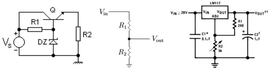
Fig. 2. On left: schematic diagram of a simple series linear regulator [2]. The regulator acts like a variable resistor making it inefficient for higher drop voltages.
